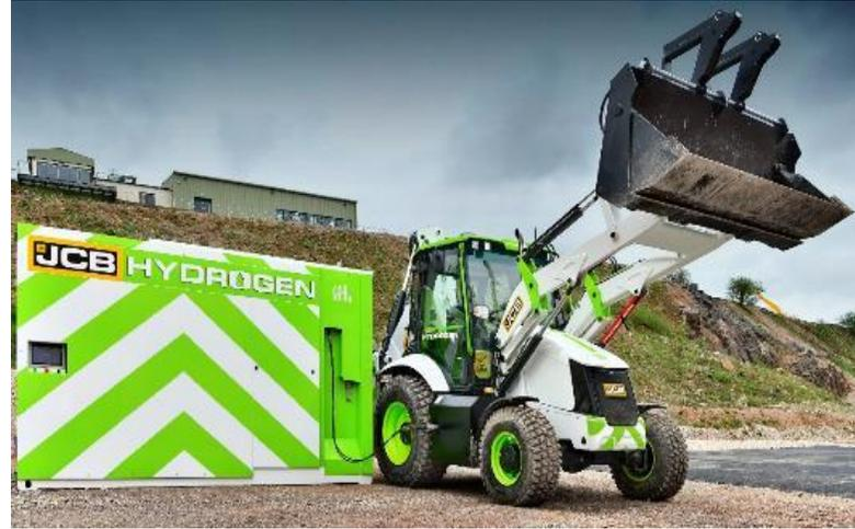
JCB Hydrogen ICE prototype loader
