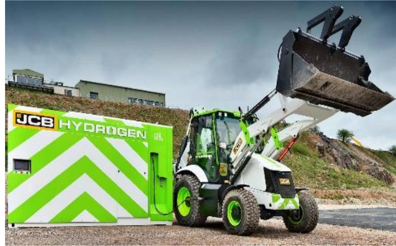
JCB Hydrogen ICE prototype loader
